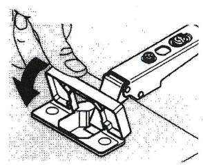
They simply push into the door and when you fold down the flap they lock into place.
