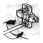
Your hinge blocks simply push into the two holes predrilled in the carcase and then tighten up the screws.
